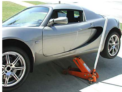
Example of secure position for jacking when using trolley jack
