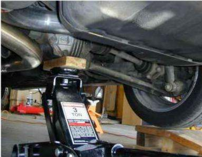
Example of secure position for jacking when using trolley jack
